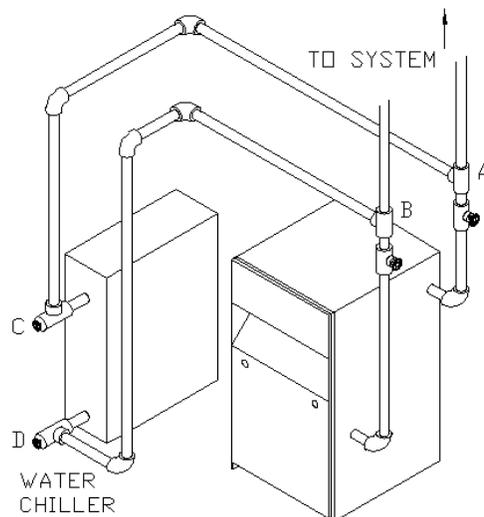
VALVES A & B OPEN FOR HEATING; CLOSE FOR COOLING
