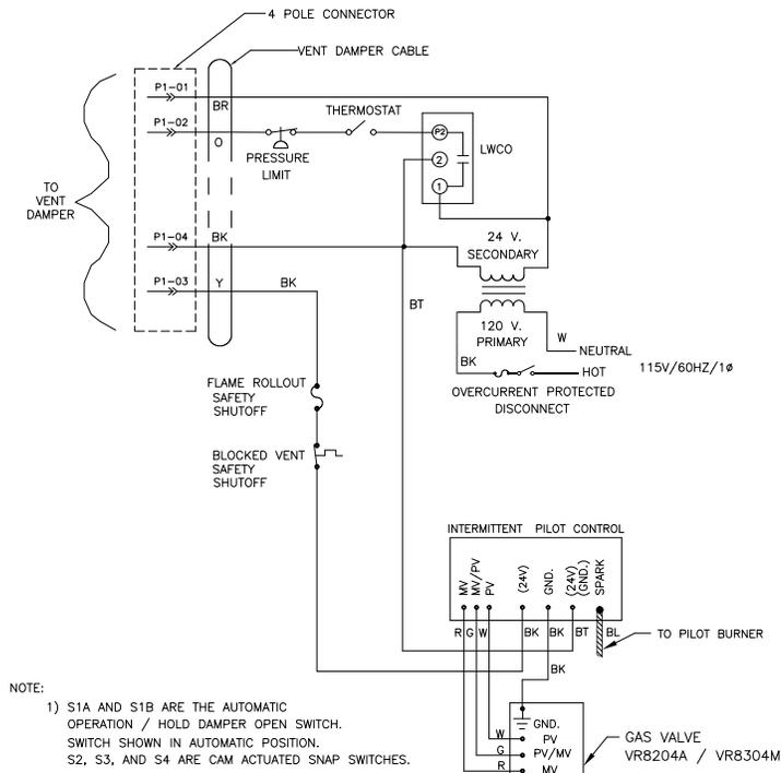
If any of the original wire as supplied with this appliance must be replaced, it must be replaced with type 105°C Thermoplastic wire or its equivalent.
