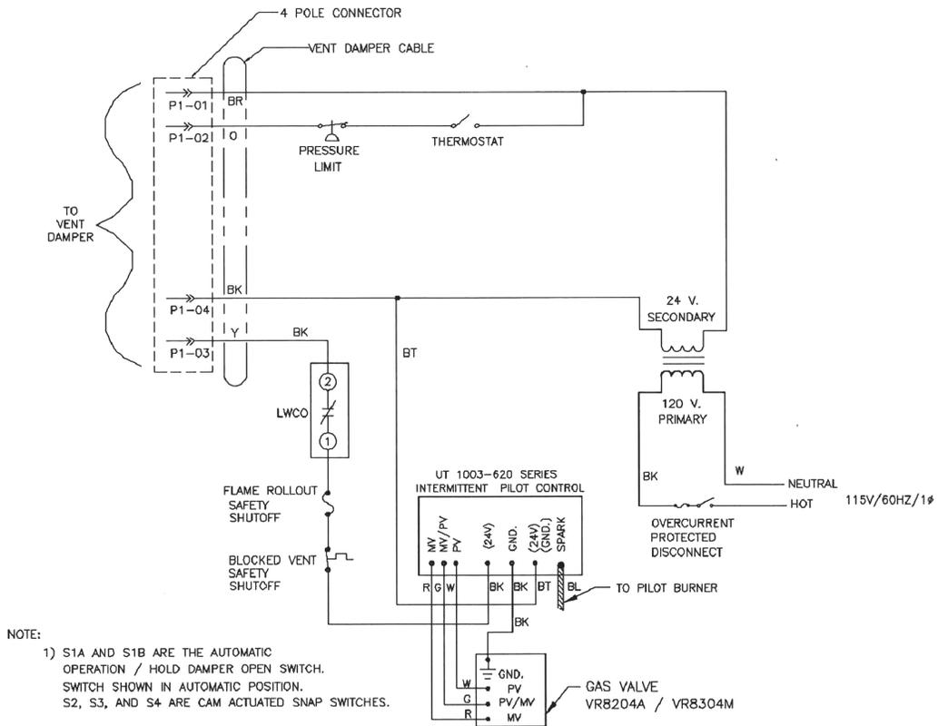
If any of the original wire as supplied with this appliance must be replaced, it must be replaced with type 105°C Thermoplastic wire or its equivalent.
