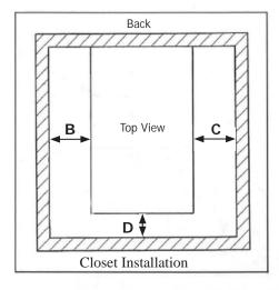
0 in /0 mm between Back of Unit and wall
