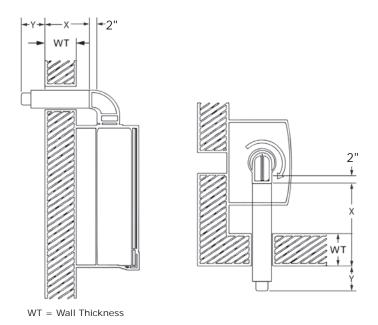
Note: 2" is insertion depth of straight pipe to elbow.
