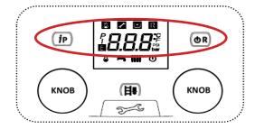
To enter the Command functions menu press (IP) and (O/R) with a long push.
