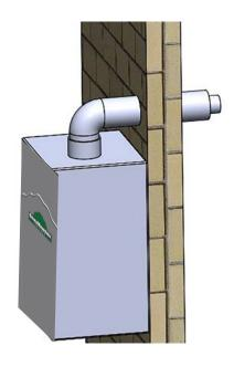
**2. Twin Pipe** – Exhaust and intake air are separate pipes, can be terminated using single wall terminals from the vent manufacturer or field built configuration using elbows or tees.
