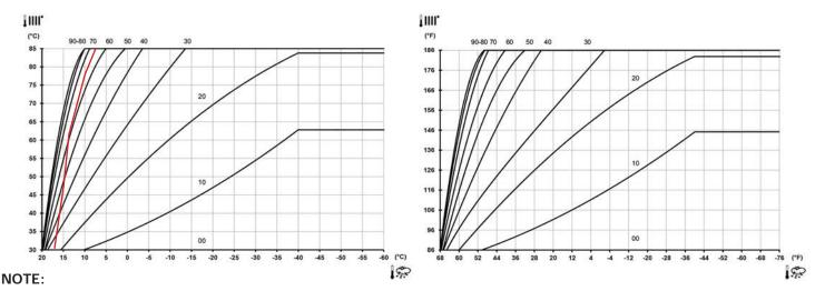
Temperatures below -40 °F (-40 °C), maximum heating flow temperature set point no longer increases, curves shown on graph become horizontal.
