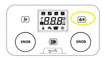
To change the boiler *MODE* press with a very short push. The mode changes are as follows:
