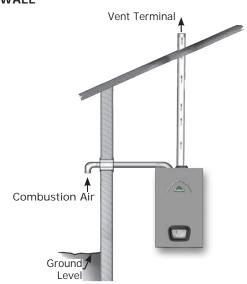
FIGURE 6-9 - TWIN PIPE FLUE ON SIDEWALL,
