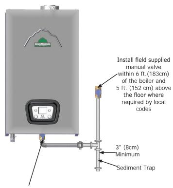
Supplied external manual main gas shutoff valve (shown in open position) with field supplied union, and sediment trap
