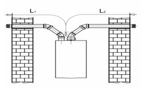
FIGURE 6-8 - TWIN PIPE ON ROOF COMBUSTION AIR ON SIDEWALL
