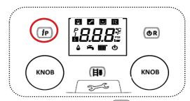
To enter in INFO menu press **iP** with a long push. This functions ends after 3 minutes, or by pressing **iP** with a long push.
