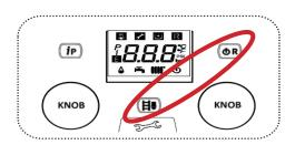
Turn Right Knob clockwise  $\P$  and increase power of the boiler at 100%.
