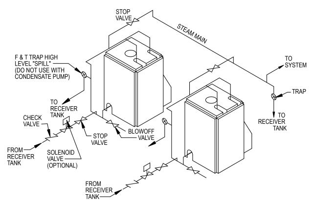
Figure #10 SUGGESTED PIPING FOR MODULAR STEAM BOILERS - GRAVITY RETURN
