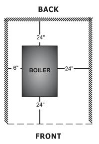
Asphyxiation, fire hazard. Do not obstruct air openings to combustion area. Follow instructions below, to maintain adequate combustion air.
