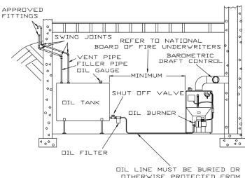
DIL LINE MUST BE BURIED DR DTHERWISE PROTECTED FROM DAMAGE. MINIMUM 3/8" IPS DR 3/8" D.D. COPPER TUBING
