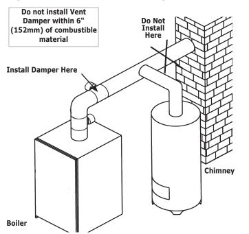
**Figure 9 - Vent Damper Position Indicator**
