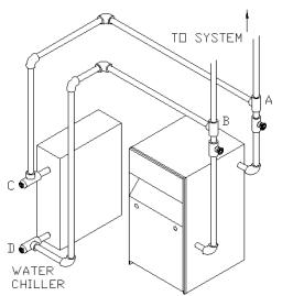
VALVES A & B OPEN FOR HEATING; CLOSE FOR COOLING
