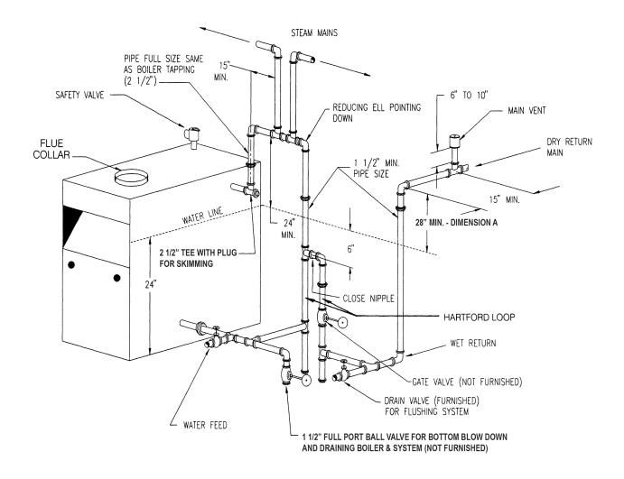
Figure 4 - Recommended Near Boiler Piping Using Two Supply Tappings [5 and 9 Sections]
