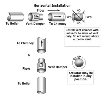
Figure 8 - Alternate Vent Damper Installation
