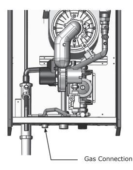
Use two (2) wrenches when tightening and fitting to pipe boiler's threaded fittings. Boiler's internal piping can be damaged if subjected to excessive torque.
