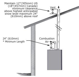
Combustion air and Vent Piping Length Page 25.
