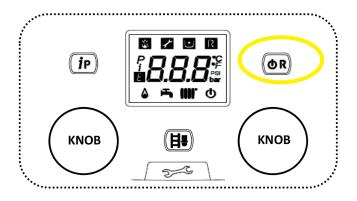
To change the boiler MODE press (O/R) with a very short push. The mode changes are as follows:
