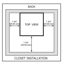
**0 in /0 mm** between the Back of the Unit and the wall
