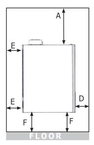
FIGURE 4-2a Service Clearances - Boiler Front
