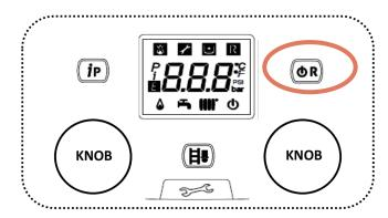
To reset the boiler press (**O/R**) with a short push (1 to 3 seconds)
