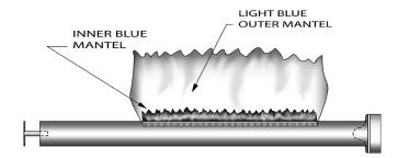
Main burner flame should form sharp blue inner mantel with no yellow.
