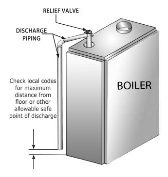
Figure 3 - Forced Hot Water Typical Piping
