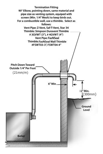
Boilers may be vented horizontally as shown in Figure 8, Page 13. Vent pipe is pitched **down** from boiler to vent termination. Do not connect other appliances to this vent.
