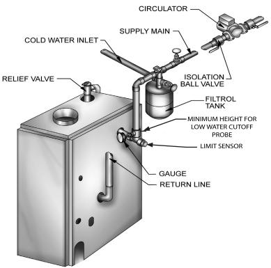
Figure 4 - Forced Hot Water Typical Piping
