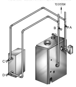
Figure 6 - Bypass Piping
