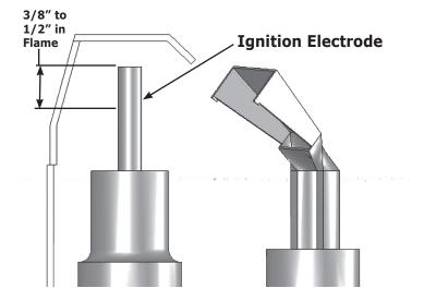
Figure 16 - Main Burner Flame
