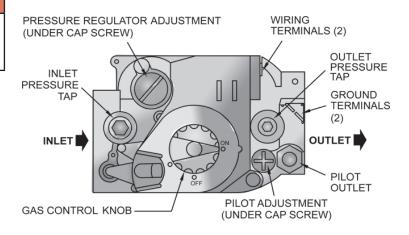
Figure 15 - Pilot Flame Adjustment
