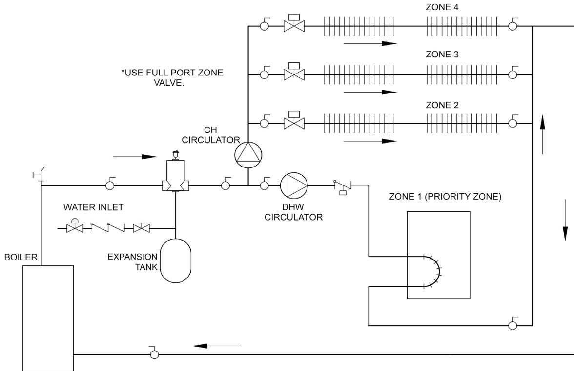
**Figure 8 - Multi-zone System With Zone Valves And DHW Priority (With Zone Valve)**
