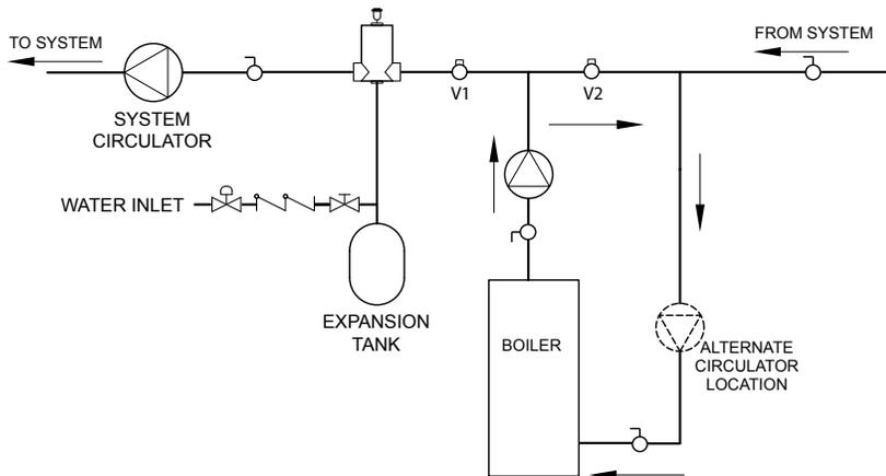
**Note:** Bypass connection not showing primary/secondary piping
