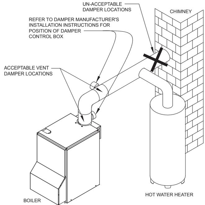
1. Verify only boiler is serviced by vent damper. See Figure 10 .
