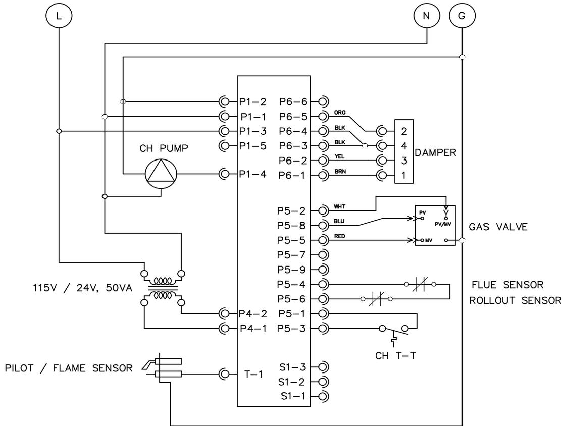
LADDER DIAGRAM: HOT WATER - ATMOSPHERIC DRAFT BOILER
