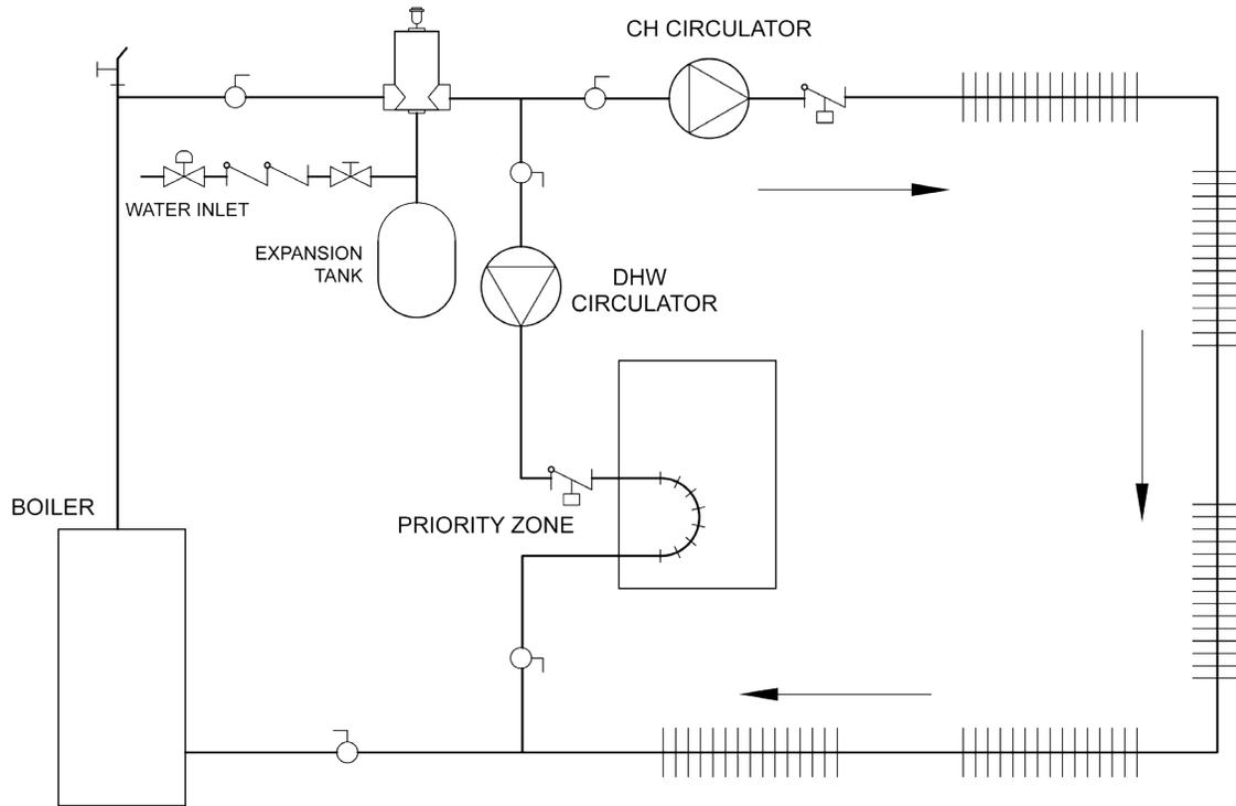
Figure 6 - Multi-Zone System with Circulators and DHW Priority
