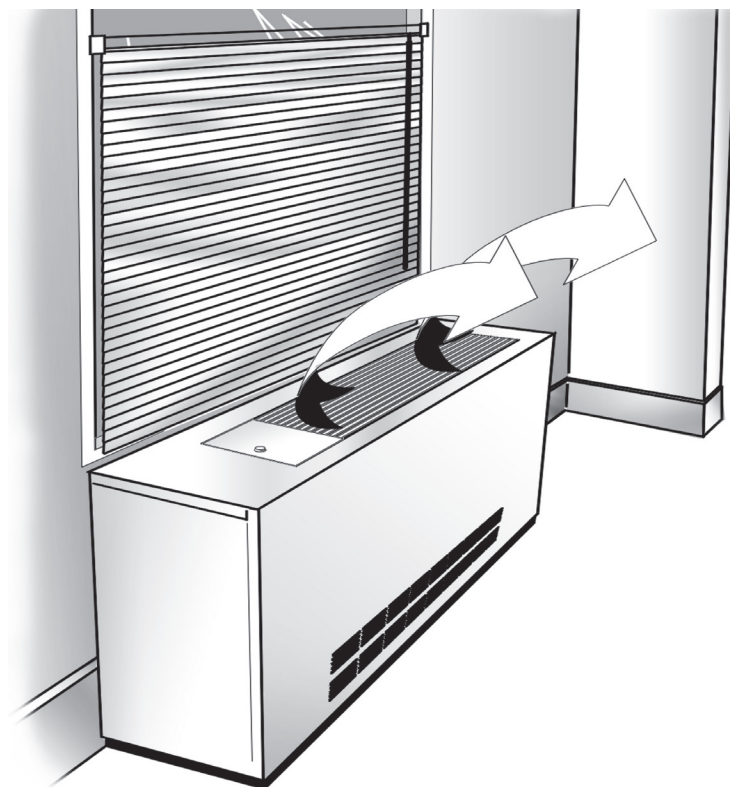
Figure 6 Proper Air Flow Example
