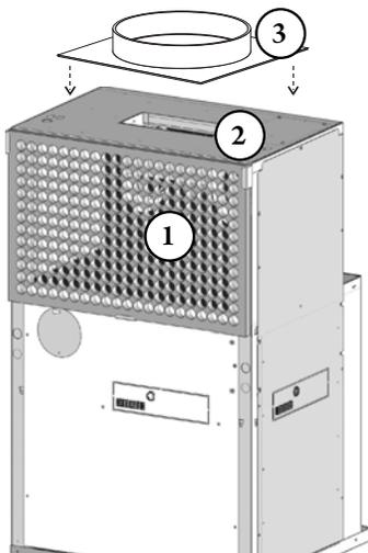
**Figure 11 Foam Gasket & Weather Angles (09–24) Front Control Panel Installations**
