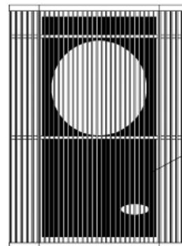
Removing the metal or plastic block-off usually only requires drilling out a few pop rivets and is generally an easy task.
