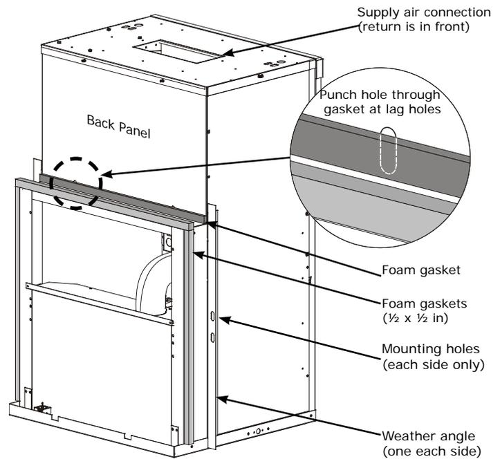
Punch holes in foam gaskets at locations of mounting holes in back panel and weather angles (see call outs in Figure 13 and Figure 14).
