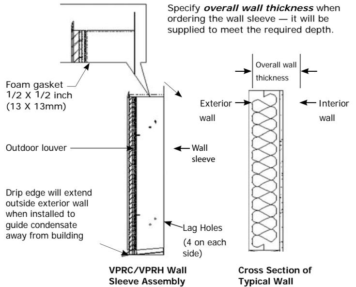
**Figure 9 Typical tabbed-assembly wall sleeve (09–24)**
