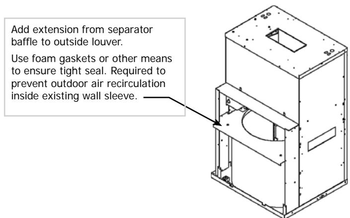
**Figure 29 Baffles On Back Of Condenser Coil**
