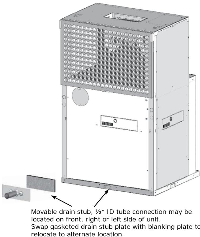
**Figure 16 Drain Stub Location (Models 30–36)**
