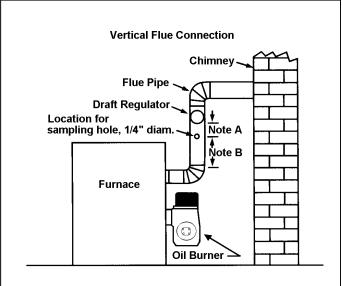
**Note A:** Locate hole at least 6 inches on the furnace side of the draft control.
