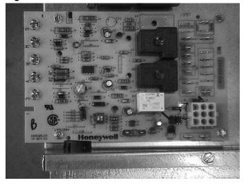
NOTE: All thermostat wires for both heating and cooling connect to the furnace at this point. A factory installed wiring harness connects the heating control functions to the R7184 oil primary control.
