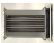
2. <u>Stainless Steel Heat Recovery Coil</u> – The large aluminum fins of the recovery coil transfer the remaining heat from the flue gases after they leave the primary heat exchanger. The stainless steel tubes are corrosion resistant and allow the flue gases to condense without causing damage to the heat exchanger.
