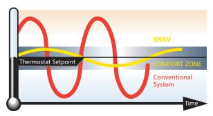
Since conventional furnaces can only operate at full capacity, they must cycle on and off when heat is required. The G95V runs for longer periods, delivering only the heat required at a slower fan speed, which drastically reduces temperature swings and increases overall comfort.
